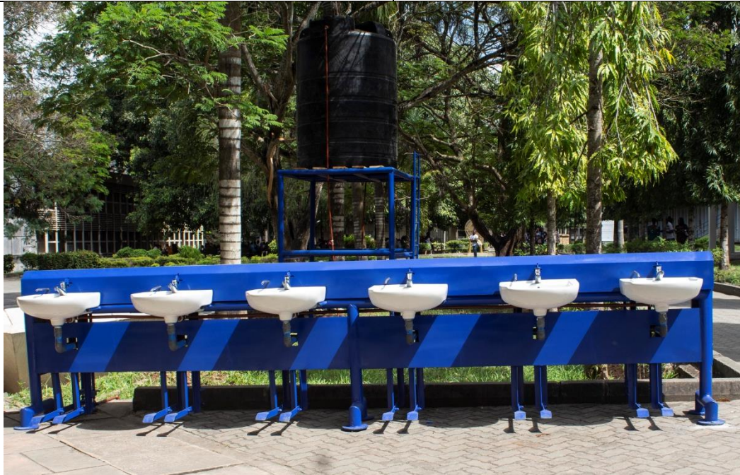
Plate 3: Foot-operated multi-facilities hand washing machine
